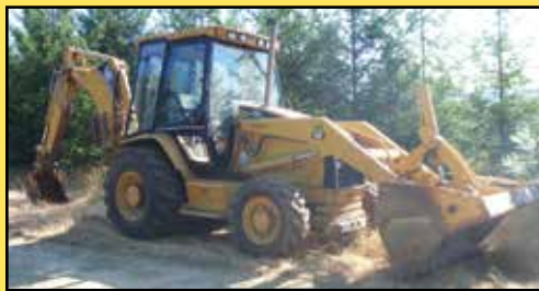
CATERPILLAR 426C TLB 4X4 4-WHEEL STEER 4-IN-1 BUCKET, AND EXTENDAHOE
