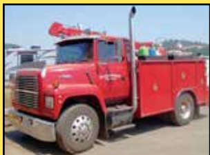
1996 FORD L7000 SERVICE TRUCK W/8,000-LB. CRANE, WELDER GENSET, AND COMPRESSOR
