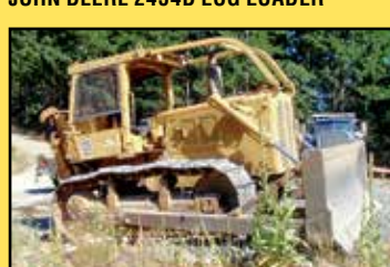
CATERPILLAR D6C W/HYSTER WINCH AND MEDFORD ARCH
